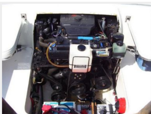
Mercuriser 5.7L Horizon- freshwater cooling
