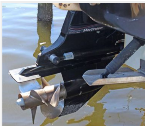
Mercruiser Bravo III Counter Rotating Outdrive
