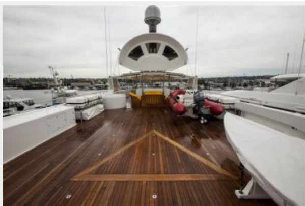
Helicopter Landing Pad, Folding Hardtop
