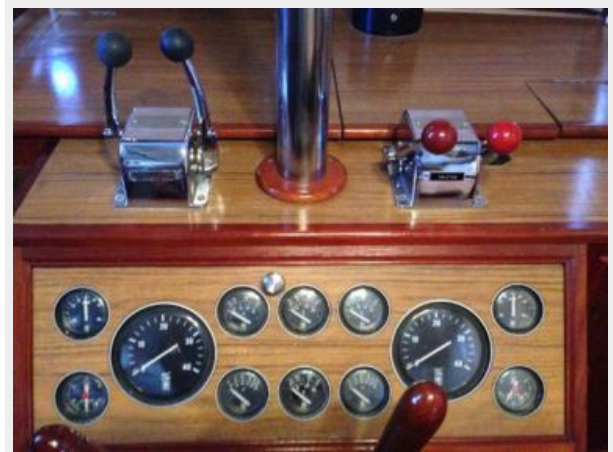
Lower Helm Controls
