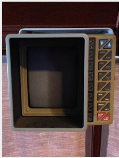
Lower Helm Radar
