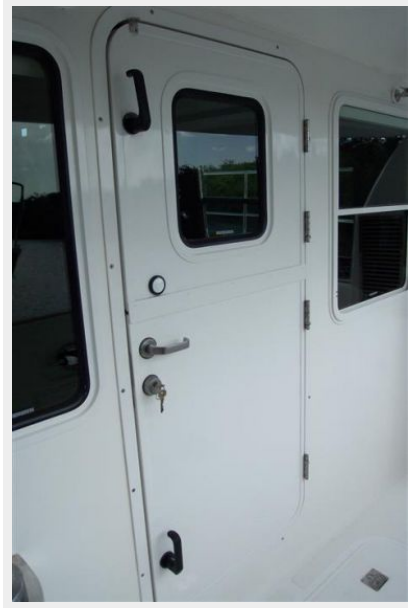
Water Tight Door to Saloon
