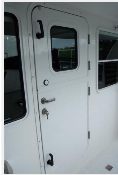
Water Tight Door to Saloon
