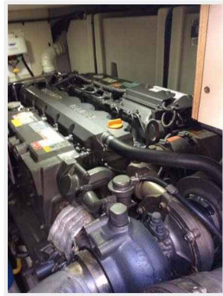
Starboard 480hp Yanmar
