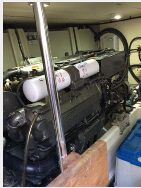
Port Engine 480hp Yanmar
