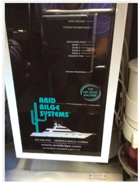
Arid Dry Bilge Vacuum System
