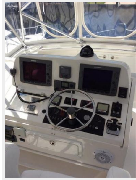
Helm Station w/ Bow & Stern Thrusters
