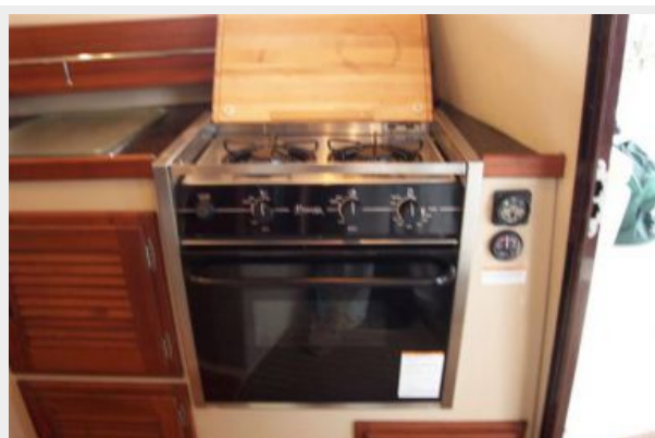
Two Burner Propane Stove/Oven
