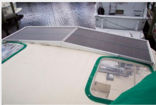
Solar Panels on Hard Top
