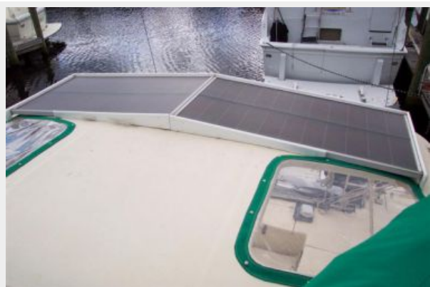
Solar Panels on Hard Top
