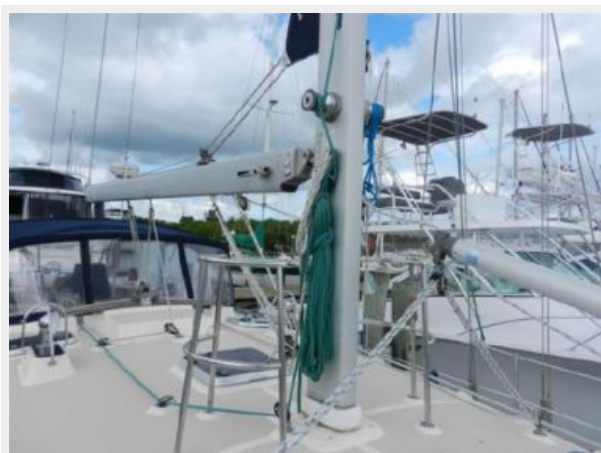
In mast furling, safety bars at mast
