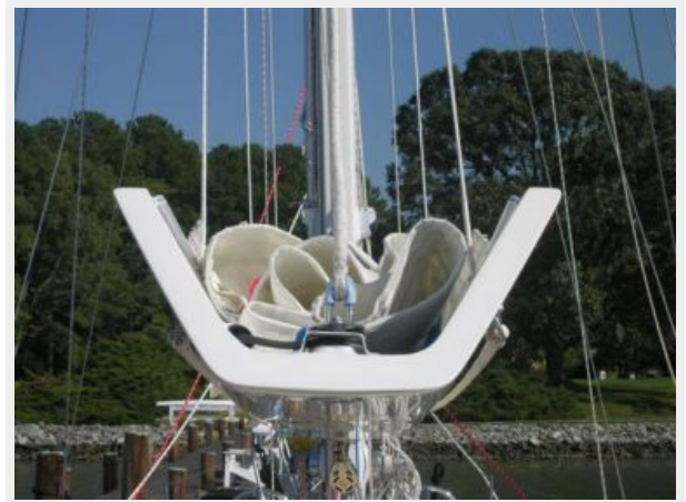
Park Avenue Boom
