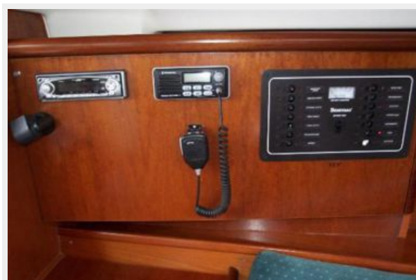
Nav Station / Electrical Panel / VHF
