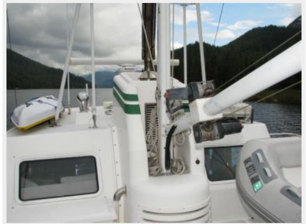
Mast and dry stack
