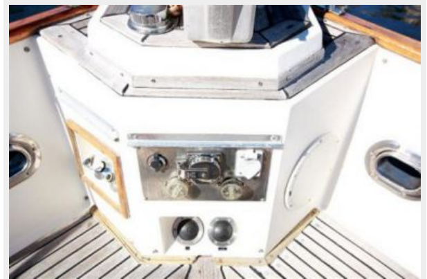
Bow electrical hookup
