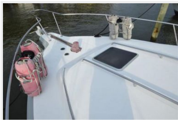
345 Sea Ray Sedan Bridge, pulpit and anchor windlass
