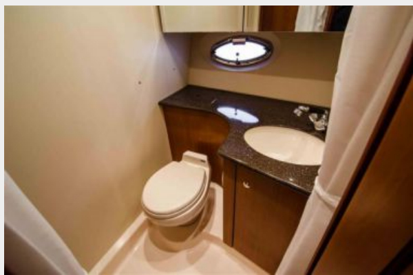
Large Head/Vacuflush System, Port Hole
