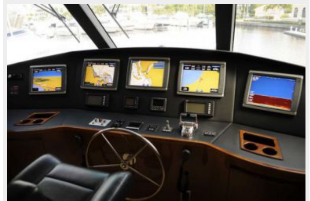
Enclosed Bridge Electronics
