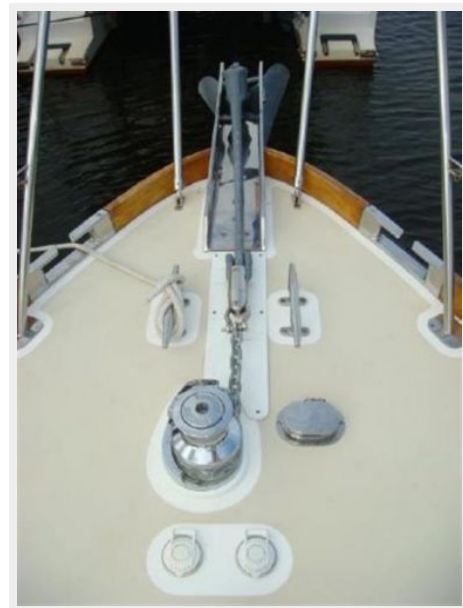
46' Alden anchor windlass
