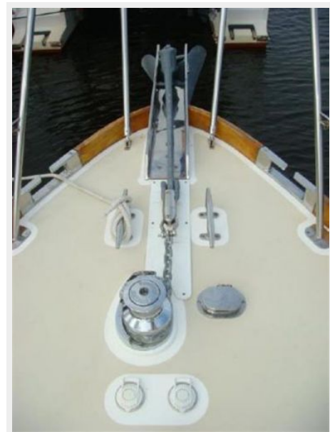
46' Alden anchor windlass
