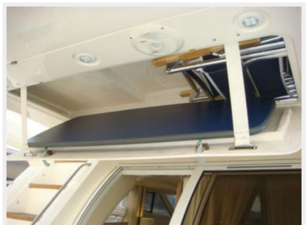
42' Sealine aftdeck overhead storage2
