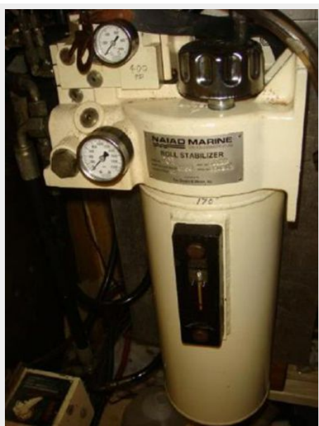
42' Kadey Krogen stabilizer system
