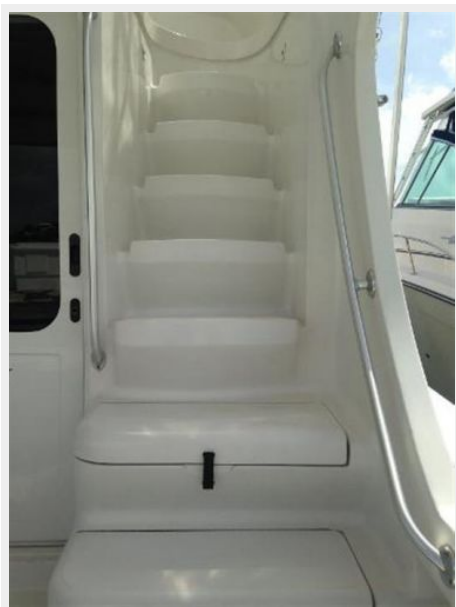
Molded Fiberglass Steps to Bridge
