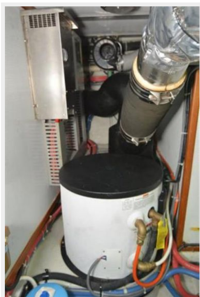
Exhaust running to port with waterlift muffler looking aft from engine room entrance
