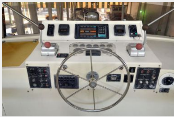
Flybridge Helm Controls
