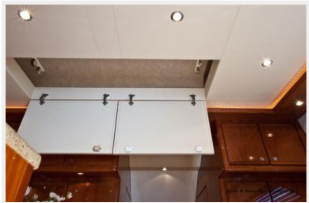
Overhead Rod Locker
