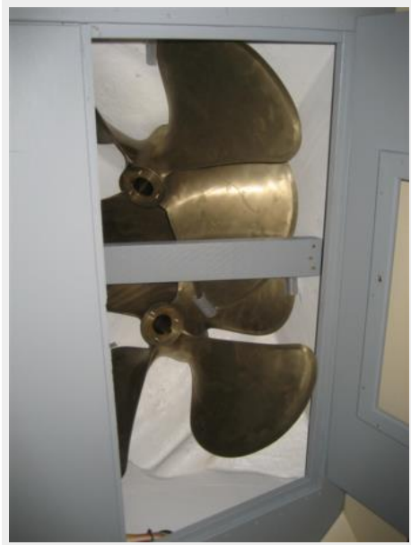
Spare Props Under VIP Berth
