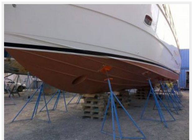
10 Year Copper Coat Bottom Job
