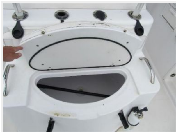
Live Well Tank
