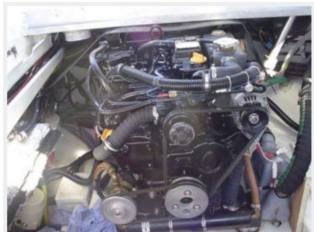
Mase/Yanmar IS9 230AC 50 htz 8.5KW Generator
