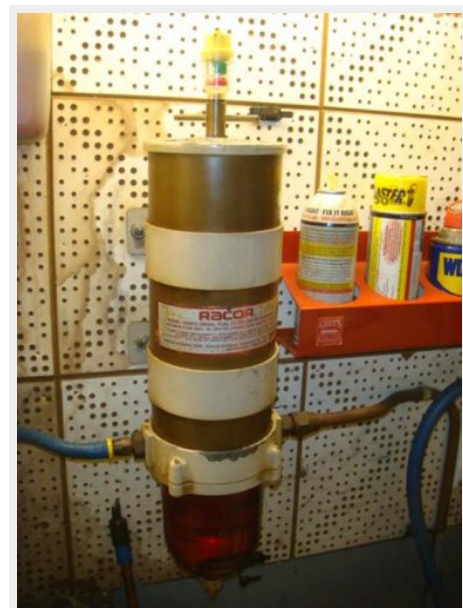
52' Jefferson starboard main engine Racor fuel filter
