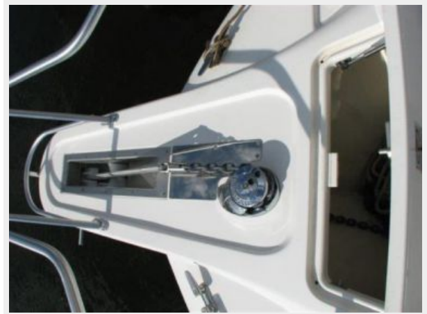
Deck 2 - Anchor Windlass & Rope Locker
