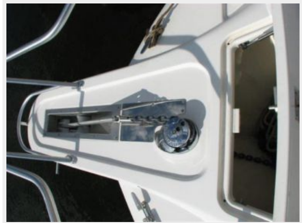
Deck 2 - Anchor Windlass & Rope Locker
