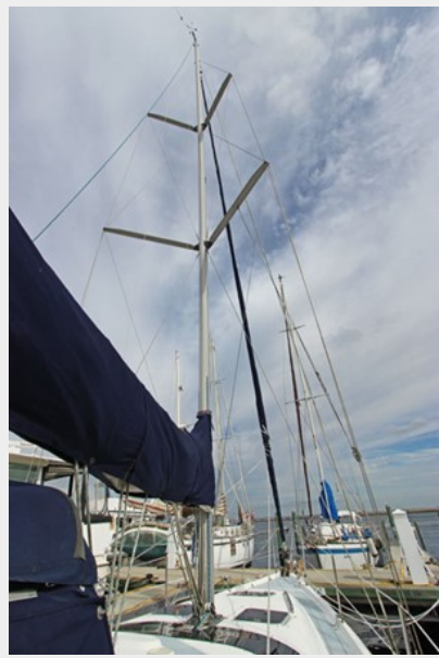
Mast View W/Double Spreaders
