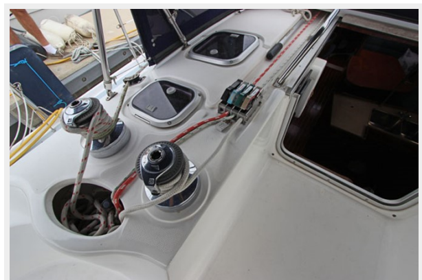
Starboard Lewmar Winches (1-44ST Primary & 1-40ST Secondary) Port Lewmar Winches (1-44ST Primary & 1-40ST Secondary)
