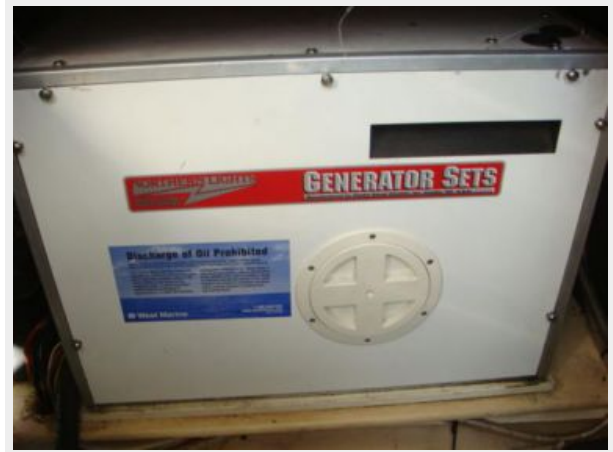
32' Nordic Tug generator sound box
