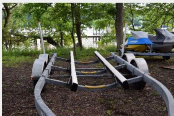
New Bunk Covers and Alignment Poles
