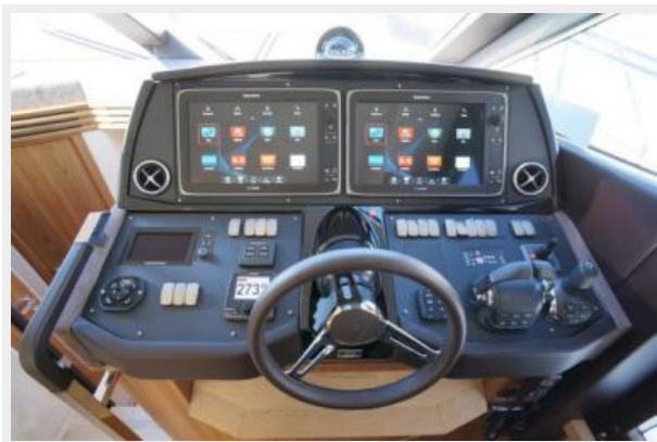
Raymarine touchscreen electronics, autopilot, Volvo joystick with Volvo DPS system
