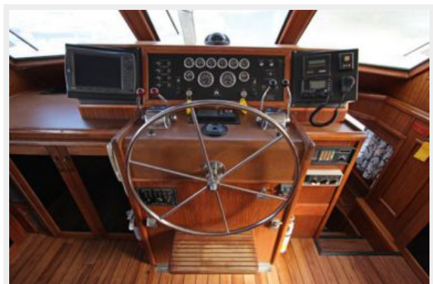
Pilothouse helm station w/Garmin 3210 plotter/sounder, Simrad AP25 autopilot, Ritchie compass, Raymarine ST60+ sounder, & ICOM IC-M504 VHF
