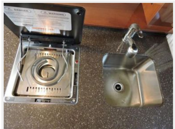
Galley Stove and Stainless Steel Sink
