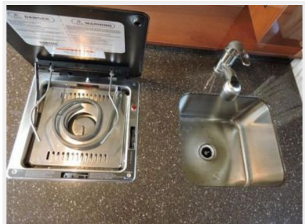
Galley Stove and Stainless Steel Sink
