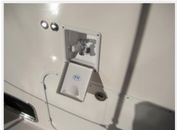
Fresh Water Outlet on Aft Deck
