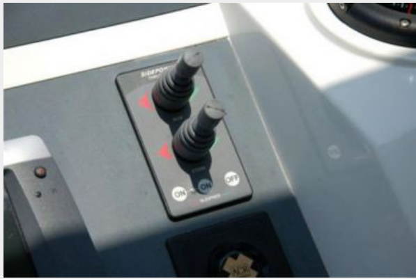
Upper Helm Thruster Controls
