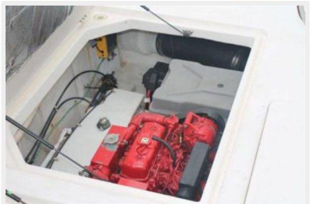
8.0 KW Westerbeke Generator
