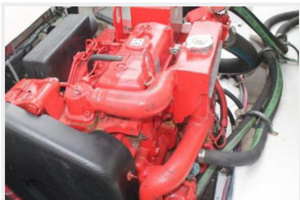
8.0 KW Westerbeke Generator
