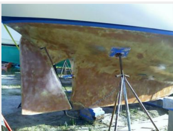
Gelcoat removed below boot stripe
