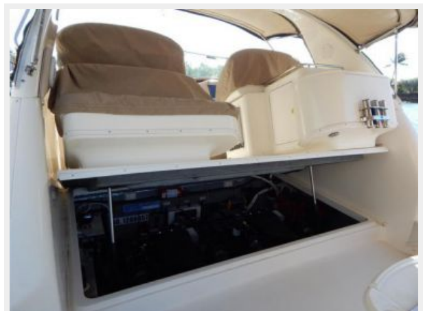
Lifting Bridge Deck
