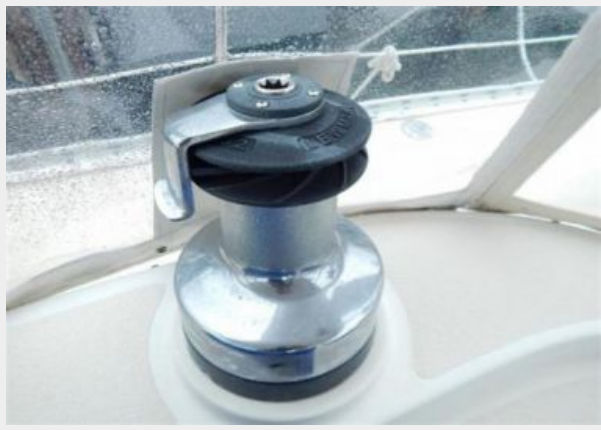
Deck Jib Winch Stbd
