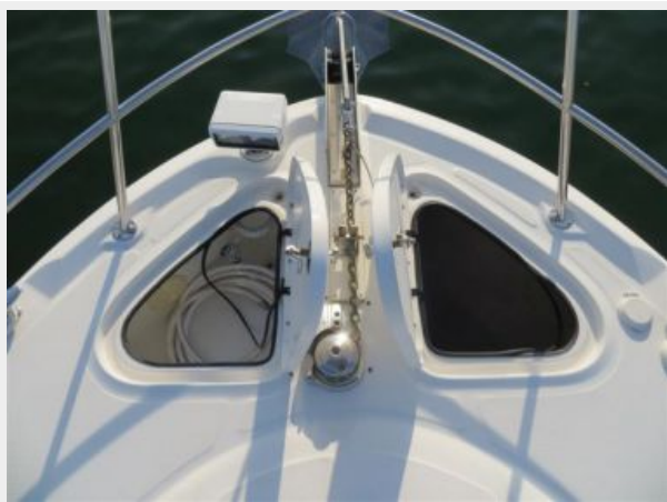
Anchor rode access
