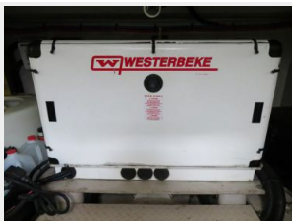
Generator sound shield
