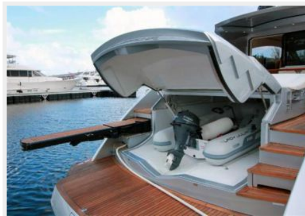
Stern Garage Tender Storage
